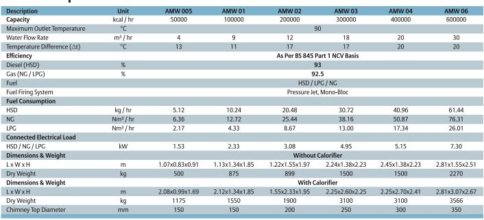
Note: Efficiency is calculated based on NCV of Diesel as 10500 kcal/kg, LPG as 24940 kcal/Nm³ and Natural Gas as 8500 kcal/Nm³. Above mentioned weight and dimensions may vary with actuals. Please refer to offer document for more details
